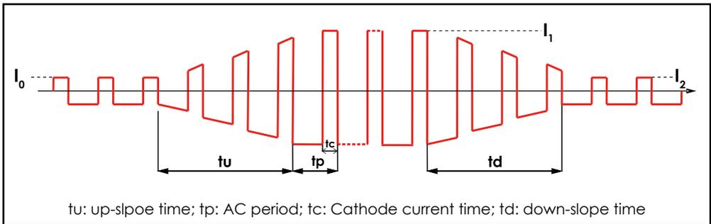
tu: up-slope time; tp: AC period; tc: Cathode current time; td: down-slope time
