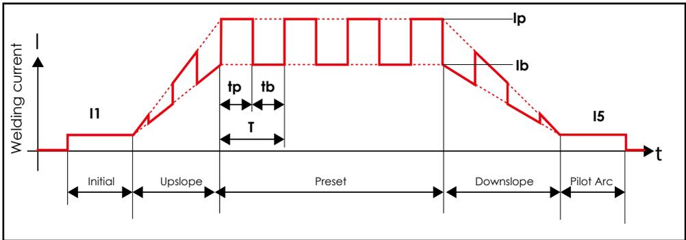
In pulsed TIG mode, all DC TIG parameters except current (I3) and another 4 adjustable parameters are available for this machine. Describe them as below.
