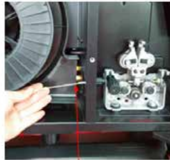
(4) Snip the wire carefully, be sure to hold the wire to prevent the spool uncoiling. Carefully feed the wire into the inlet guide tube of the wire feed unit.
